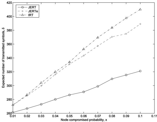
Fig. 12. Comparing the expected number of transmitted symbols in the JERT scheme and related schemes, with  $(n, k) = (1,023,255)$ .
