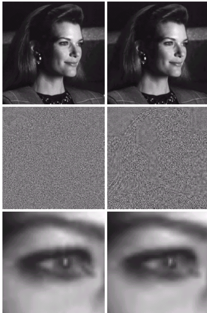
FIGURE 8.40 (a), (c), and (e) Wavelet coding results comparable to the transform-based results in Figs. 8.38(a), (c), and (e); (b), (d), and (f) similar results for Figs. 8.38(b), (d), and (f).
