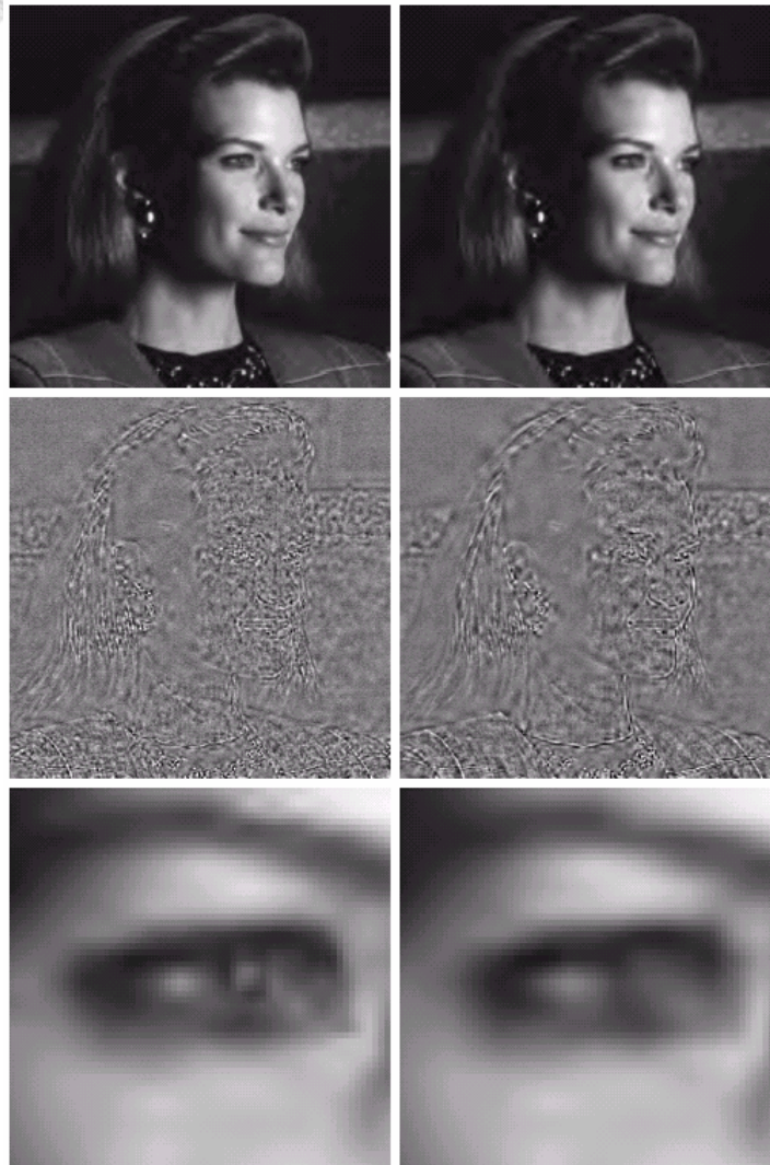
FIGURE 8.41 (a), (c), and (e) Wavelet coding results with a compression ratio of 108 to 1; (b), (d), and (f) similar results for a compression of 167 to 1.
