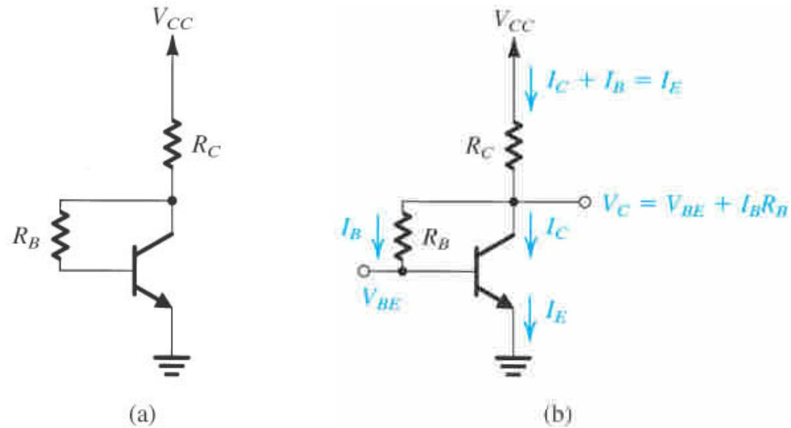
**Figure 5.46** (a) A common-emitter transistor amplifier biased by a feedback resistor  $R_B$ . (b) Analysis of the circuit in (a).
