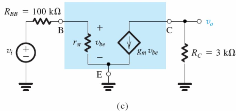
**FIGURE 5.53** Example 5.14: (a) circuit; (b) dc analysis; (c) small-signal model.
