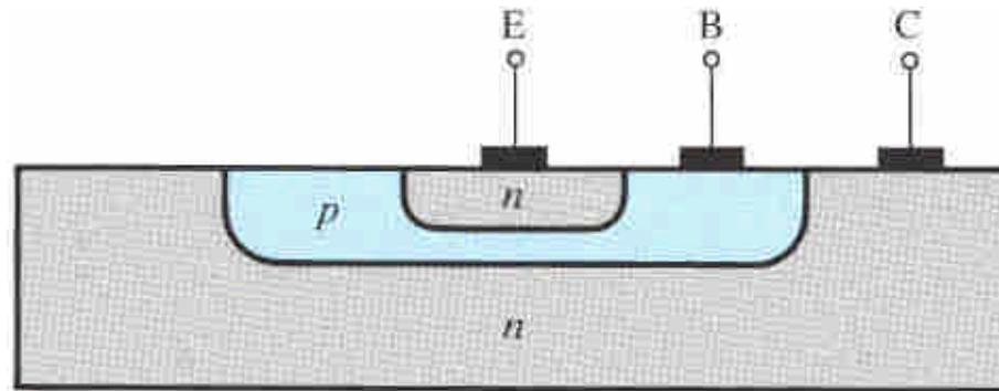
**Figure 5.6** Cross-section of an *npn* BJT.
