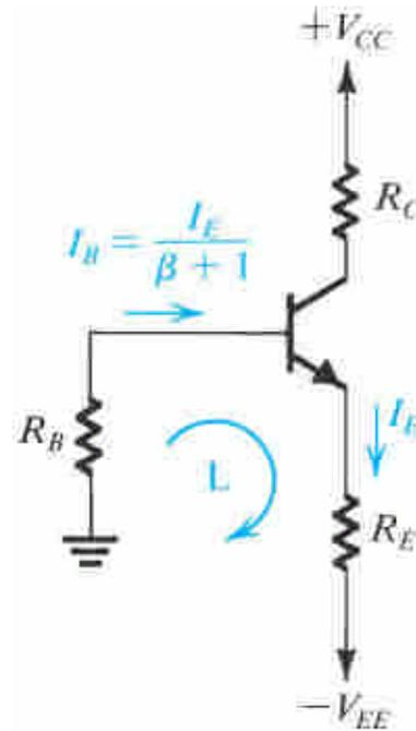
**Figure 5.45** Biasing the BJT using two power supplies. Resistor  $R_B$  is needed only if the signal is to be capacitively coupled to the base. Otherwise, the base can be connected directly to ground, or to a grounded signal source, resulting in almost total  $\beta$ -independence of the bias current.
