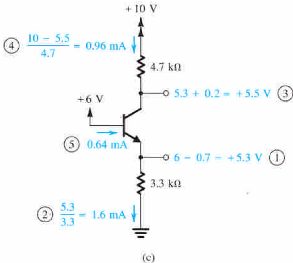
**FIGURE 5.35** Analysis of the circuit for Example 5.5. Note that the circled numbers indicate the order of the analysis steps.
