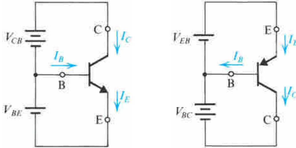
**Figure 5.14** Voltage polarities and current flow in transistors biased in the active mode.
