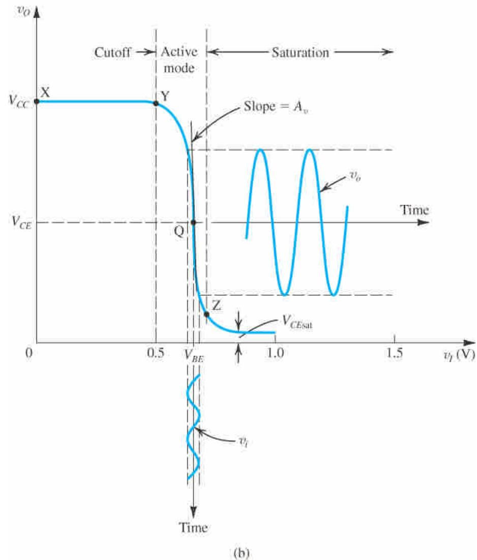
**Figure 5.26** (a) Basic common-emitter amplifier circuit. (b) Transfer characteristic of the circuit in (a). The amplifier is biased at a point Q, and a small voltage signal  $v_i$  is superimposed on the dc bias voltage  $V_{BE}$ . The resulting output signal  $v_o$  appears superimposed on the dc collector voltage  $V_{CE}$ . The amplitude of  $v_o$  is larger than that of  $v_i$  by the voltage gain  $A_v$ .
