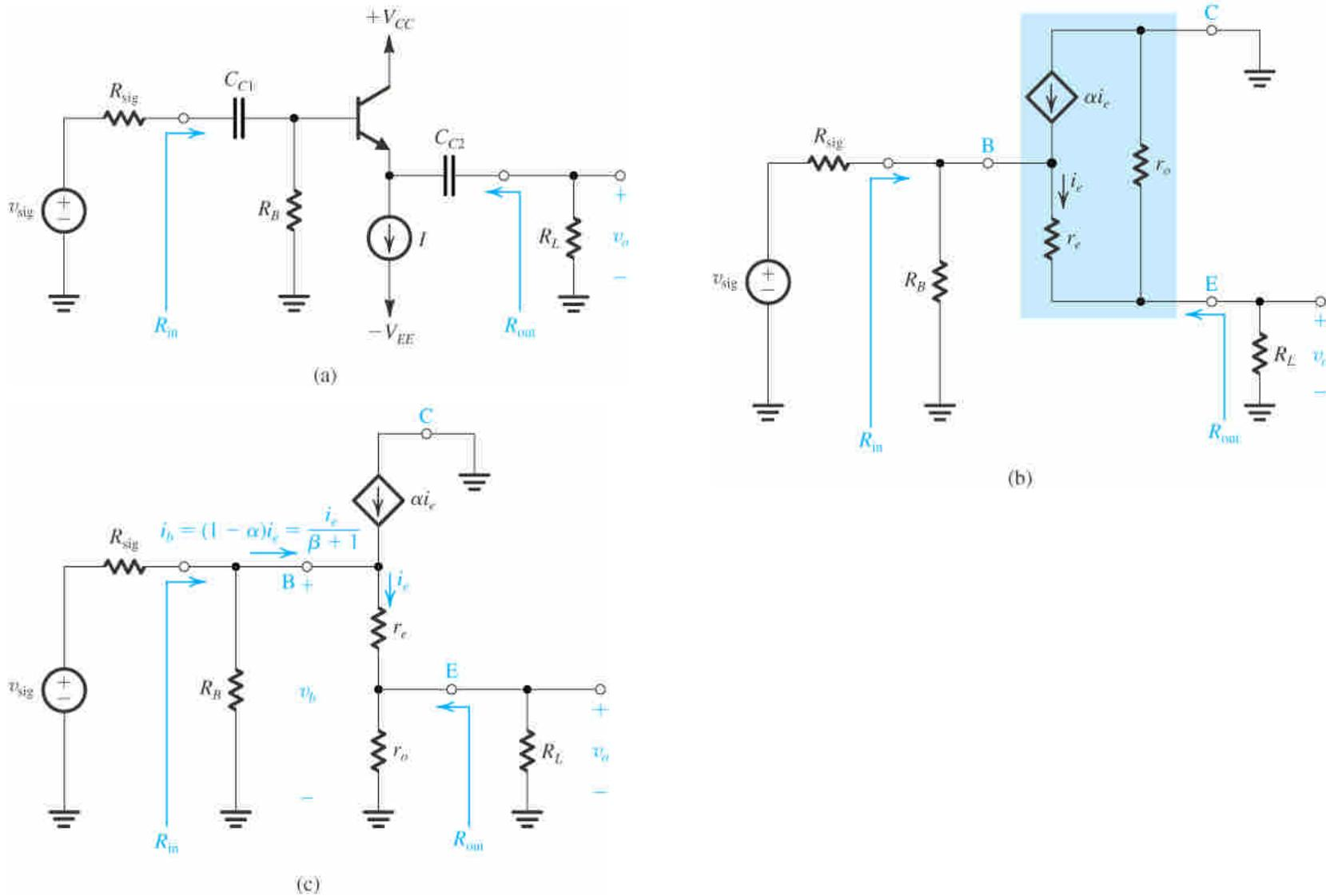
**Figure 5.63** (a) An emitter-follower circuit based on the structure of Fig. 5.59. (b) Small-signal equivalent circuit of the emitter follower with the transistor replaced by its T model augmented with  $r_o$ . (c) The circuit in (b) redrawn to emphasize that  $r_o$  is in parallel with  $R_L$ . This simplifies the analysis considerably.
