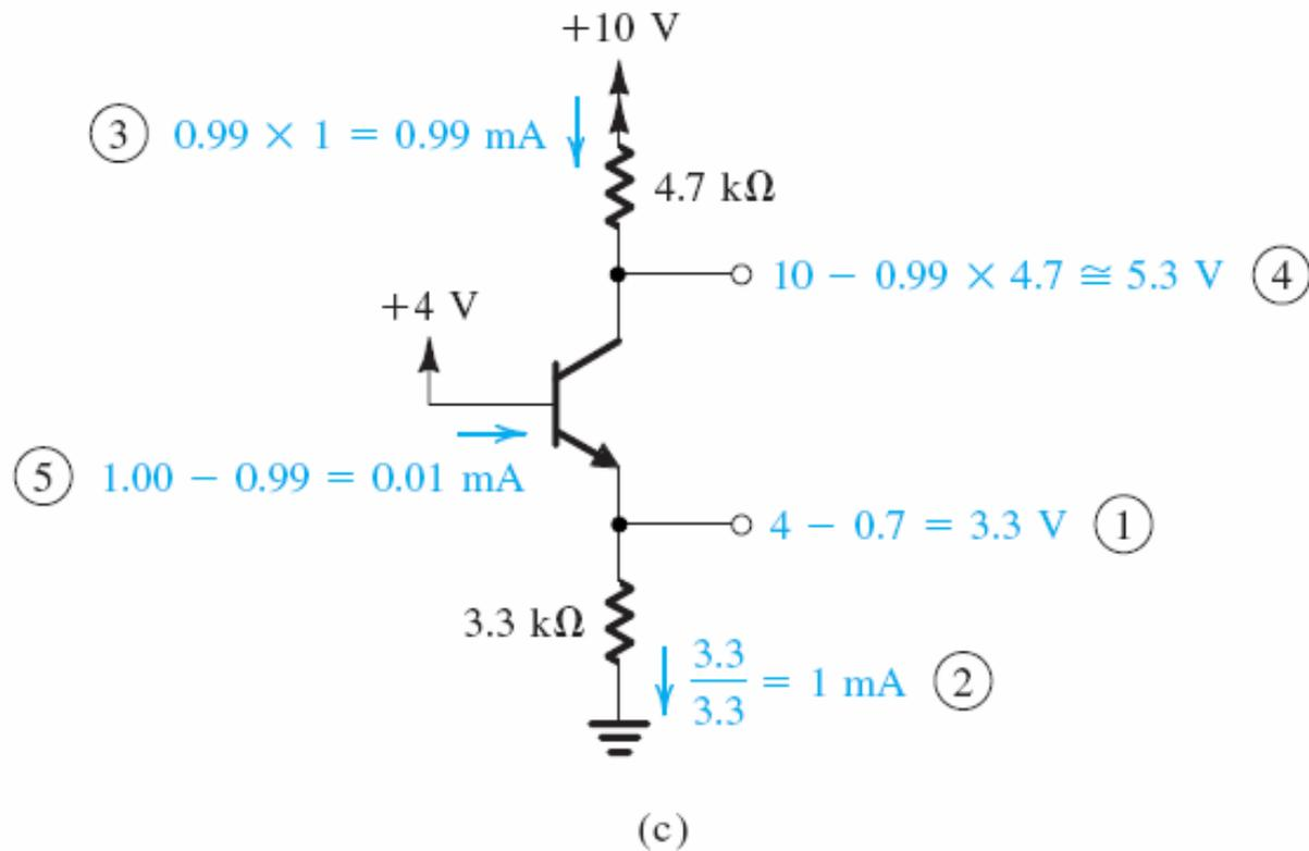
**FIGURE 5.34** Analysis of the circuit for Example 5.4: (a) circuit; (b) circuit redrawn to remind the reader of the convention used in this book to show connections to the power supply; (c) analysis with the steps numbered.
