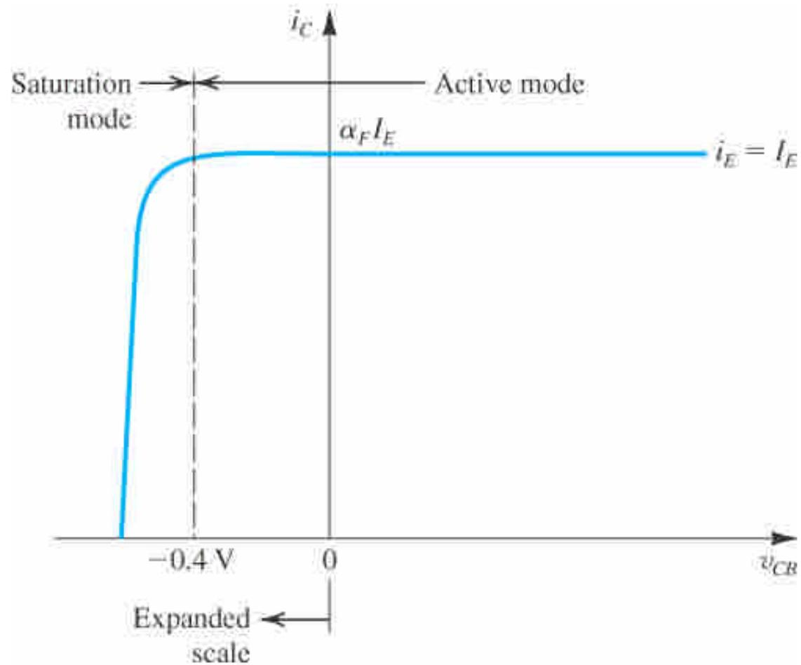
**Figure 5.9** The  $i_C$ - $v_{CB}$  characteristic of an *npn* transistor fed with a constant emitter current  $I_E$ . The transistor enters the saturation mode of operation for  $v_{CB} < -0.4$  V, and the collector current diminishes.
