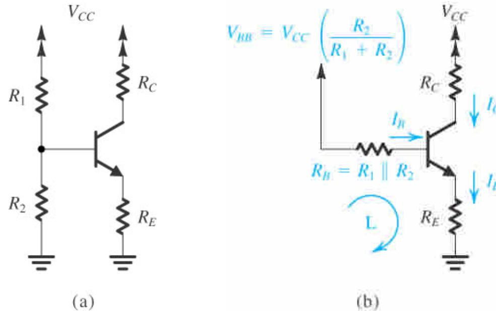
**Figure 5.44** Classical biasing for BJTs using a single power supply: (a) circuit; (b) circuit with the voltage divider supplying the base replaced with its Thévenin equivalent.
