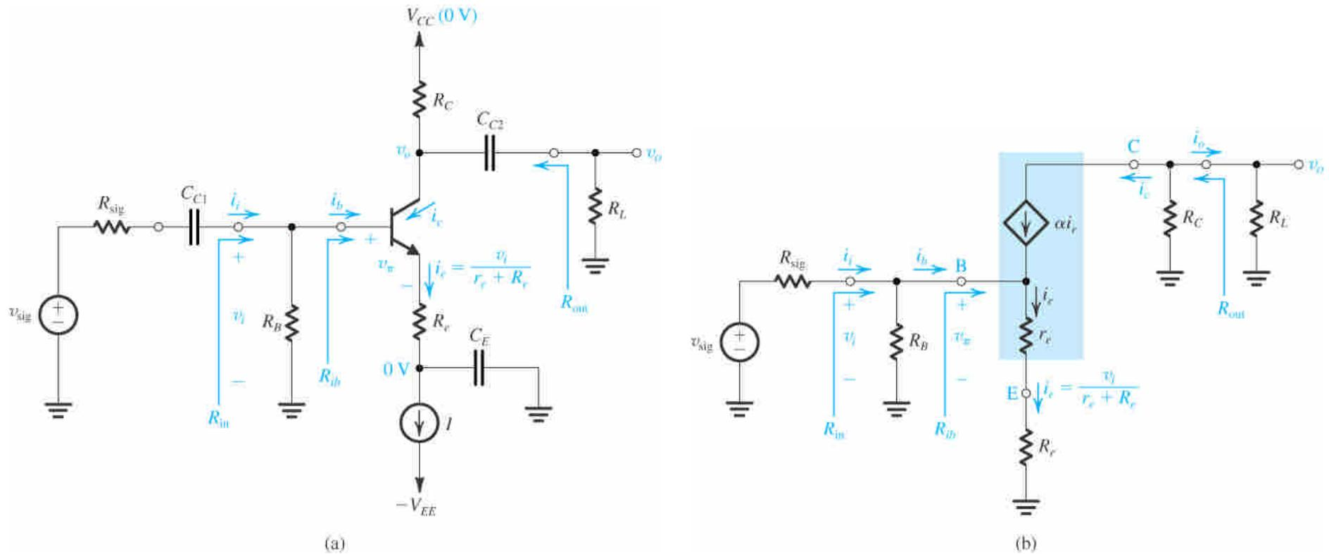
**Figure 5.61** (a) A common-emitter amplifier with an emitter resistance  $R_e$ . (b) Equivalent circuit obtained by replacing the transistor with its T model.
