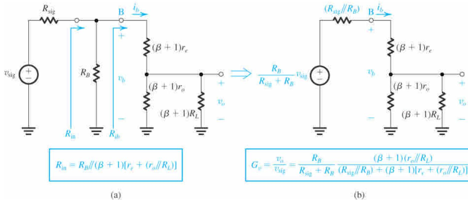
**Figure 5.64** (a) An equivalent circuit of the emitter follower obtained from the circuit in Fig. 5.63(c) by reflecting all resistances in the emitter to the base side. (b) The circuit in (a) after application of Thévenin theorem to the input circuit composed of  $v_{sig}$ ,  $R_{sig}$ , and  $R_B$ .
