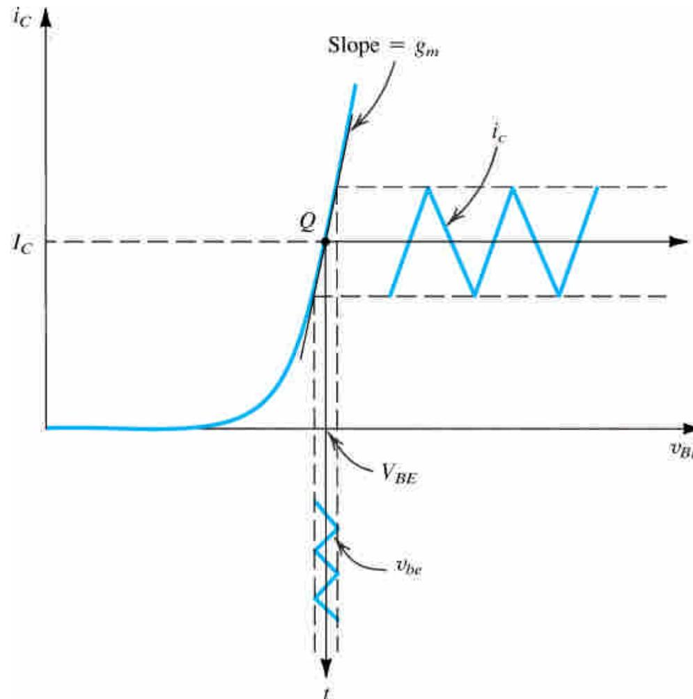
**Figure 5.49** Linear operation of the transistor under the small-signal condition: A small signal  $v_{be}$  with a triangular waveform is superimposed on the dc voltage  $V_{BE}$ . It gives rise to a collector signal current  $i_c$ , also of triangular waveform, superimposed on the dc current  $I_C$ . Here,  $i_c = g_m v_{be}$ , where  $g_m$  is the slope of the  $i_C$ - $v_{BE}$  curve at the bias point  $Q$ .
