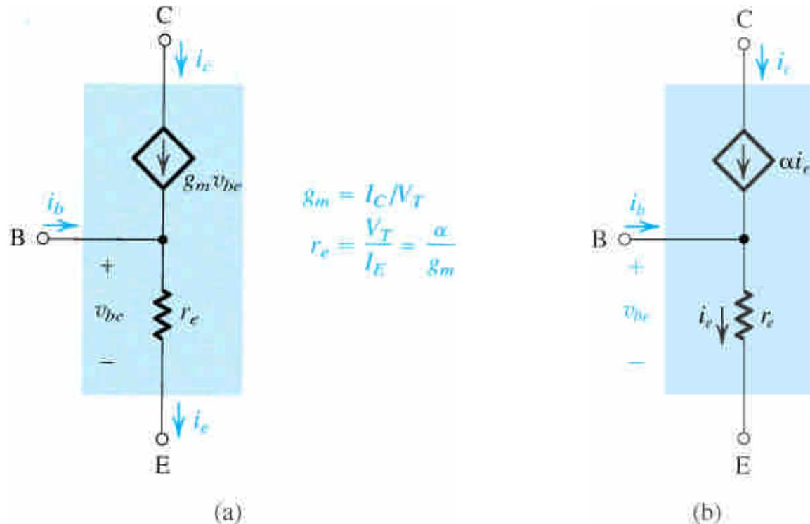
**Figure 5.52** Two slightly different versions of what is known as the *T model* of the BJT. The circuit in (a) is a voltage-controlled current source representation and that in (b) is a current-controlled current source representation. These models explicitly show the emitter resistance  $r_e$  rather than the base resistance  $r_\pi$  featured in the hybrid- $\pi$  model.
