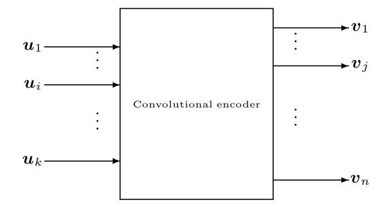
1. The encoders of convolutional codes can be represented by *linear* time-invariant (LTI) systems.
