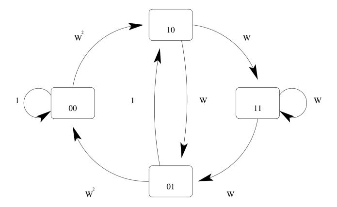
1. The power of the operator W corresponds to the Hamming weight of the code block associated with the transition.
