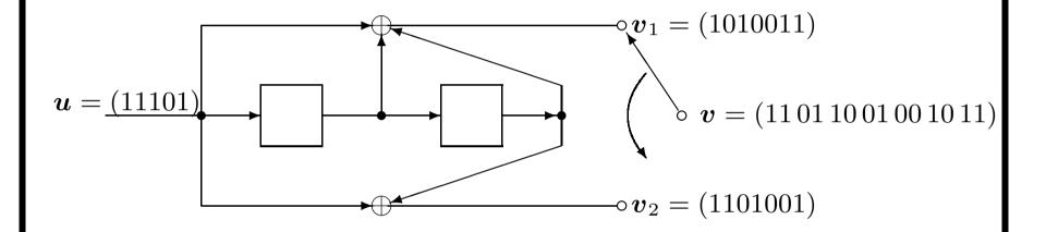
$$egin{array}{lll} oldsymbol{g}_1 &=& (1,1,1,0,\ldots) = (1,1,1), \ oldsymbol{g}_2 = (1,0,1,0,\ldots) = (1,0,1) \ oldsymbol{v}_1 &=& (1,1,1,0,1)*(1,1,1) = (1,0,1,0,0,1,1) \ oldsymbol{v}_2 &=& (1,1,1,0,1)*(1,0,1) = (1,1,0,1,0,0,1) \end{array}$$
